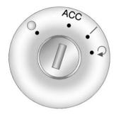
The ignition switch has four different positions.
